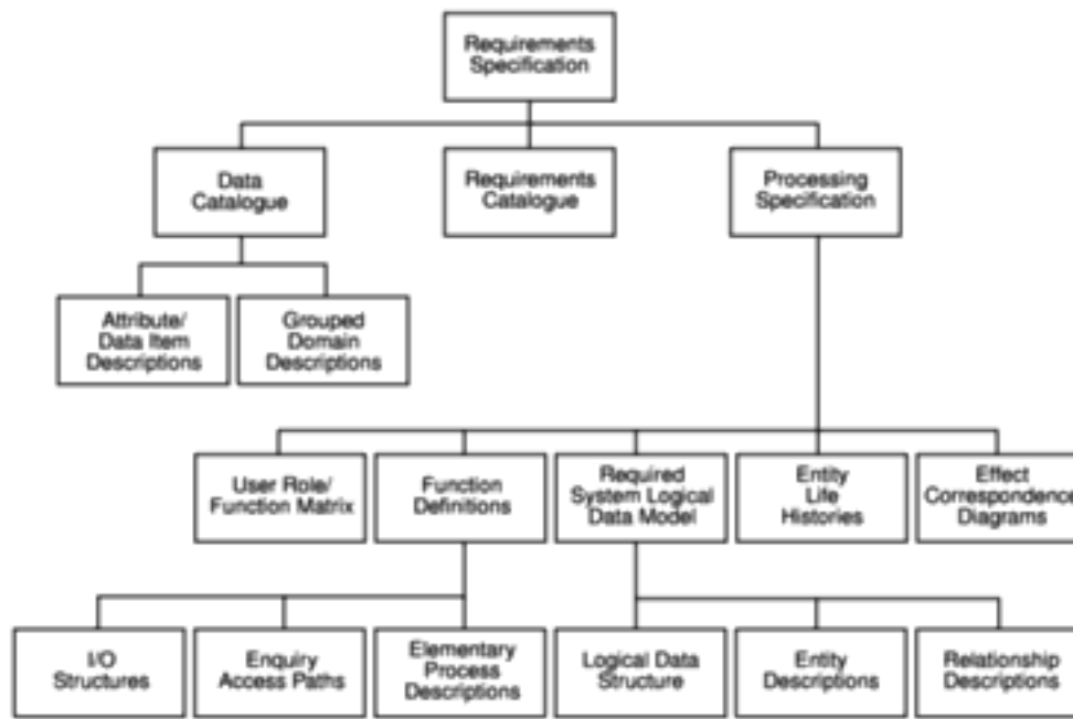
Figure 6.3 SSADM Product Breakdown Structure for Requirements Specification (adapted from Goodland and Slater).
