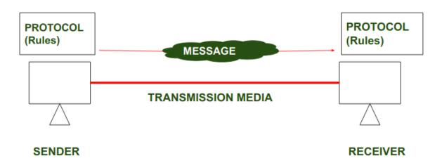
In above diagrams Protocols are shown as set of rules . Such that Communication between Sender and Receiver is not possible without Protocol.
