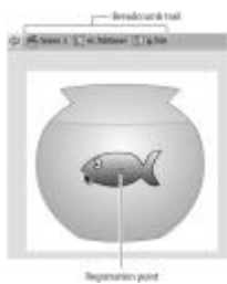
Figure 24a Flash is in editing-in-place mode for a graphic symbol called g_fish , which is inside a movie clip called m_fishbowl . The breadcrumb trail leads back to the original contents of the stage.
