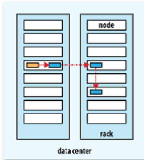
Figure: A typical replica pipeline
