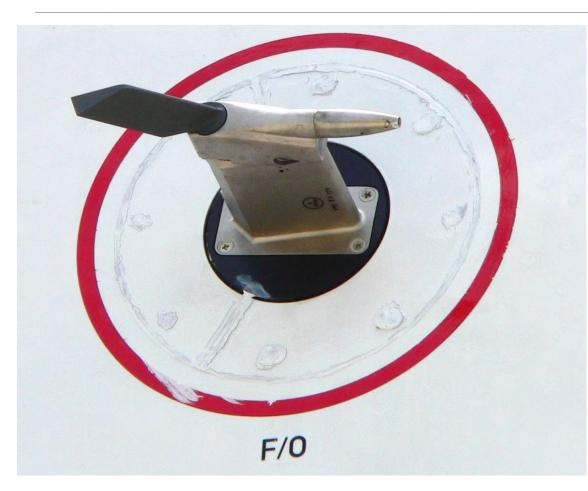
To measure the IAS, aircraft are fitted with a sensor called a <u>Pitot tube</u>. The Pitot tube is a tube that is exposed to the airflow and can measure the **total pressure** exerted on the air<u>craft</u>.
