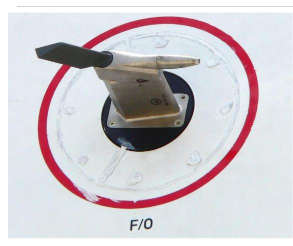
To measure the IAS, aircraft are fitted with a sensor called a <u>Pitot tube</u>. The Pitot tube is a tube that is exposed to the airflow and can measure the **total pressure** exerted on the aircraft.
