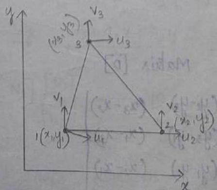
$$\text{Displacement } \{u\} = \begin{Bmatrix} u_1 \\ u_2 \\ u_3 \\ v_1 \\ v_2 \\ v_3 \end{Bmatrix} \begin{array}{l} \rightarrow x \text{ direction} \\ \rightarrow y \text{ direction} \end{array}$$
