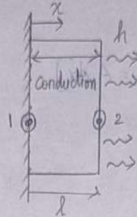
Consider a One Dimensional element with Nodes 1 and 2.  $T_1$  and  $T_2$  are the temperatures at the respective Nodes. Assume convection occurs from only right end of the element.
