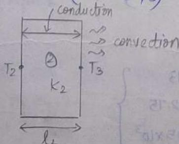
This element consists of both conduction and convection
