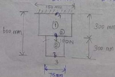
$$\begin{aligned} \text{Area at node 1} &= \text{Width} \times \text{Thickness} \\ &= 150 \times 25 \\ &= 3750 \text{ mm}^2 \end{aligned}$$
