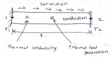
consider a rod with nodes , and z. This rod Subjected to conduction, convection and Internal heat generalizar.
