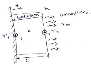
consider a one dimensional element with nodes, and . T, and Tz are the temperatures at the respective nodes. Assume convection occurs only from the right end of the element.
