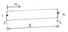
Consider box element with nodes 1 and 2.  $T_1, T_2$  are the temperature at the respective nodes. So,  $T_1$  and  $T_2$  are considered as DOF of this box element.
