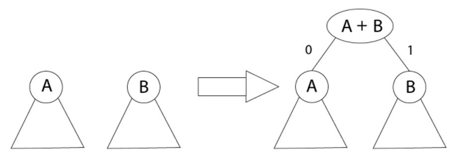
The algorithm builds the tree T analogous to the optimal code in a bottom-up manner. It starts with a set of |C| leaves (C is the number of characters) and performs |C| - 1 'merging' operations to create the final tree. In the Huffman algorithm 'n' denotes the quantity of a set of characters, z indicates the parent node, and x & y are the left & right child of z respectively.
