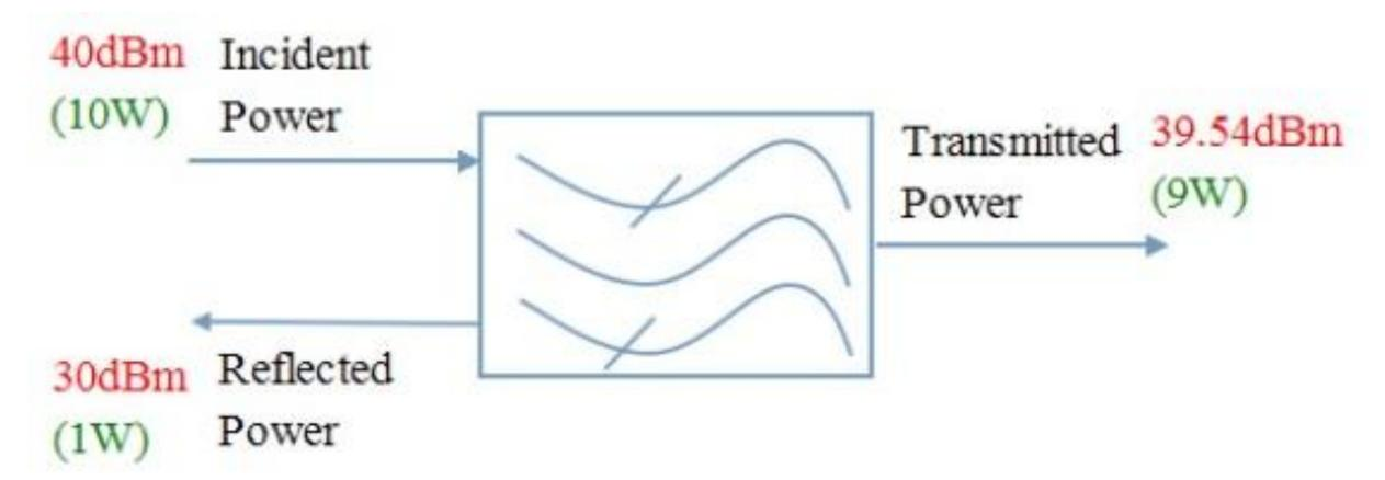
•Insertion Loss = 40dBm - 39.54dBm = 0.46dB
