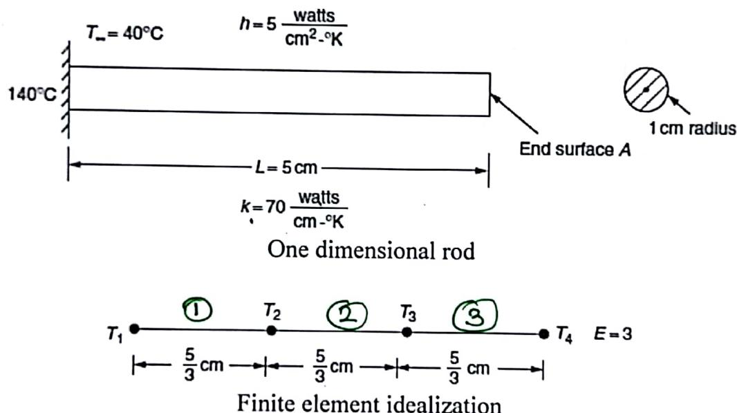
For elements (1) and (2) in the situation, the conductance and thermal load matrix area given by
