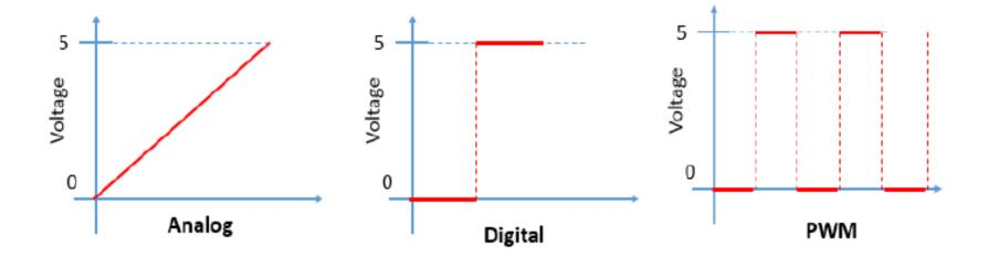
Difference between Analog, Digital and PWM Pins
