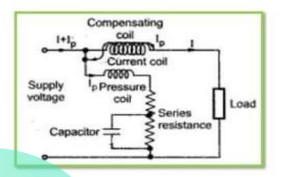
the pressure coil inductance introduces error whose magnitude is given by VI sin  $\phi$  tan  $\beta$ . If power factor is low then  $\phi$ is large and hence sin  $\phi$  is large. Thus the error introduced in the measurement is appreciable which must be compensated. It is compensated by connecting a capacitor across a part of series resistance in the pressure coil circuit which is shown in the Fig.
