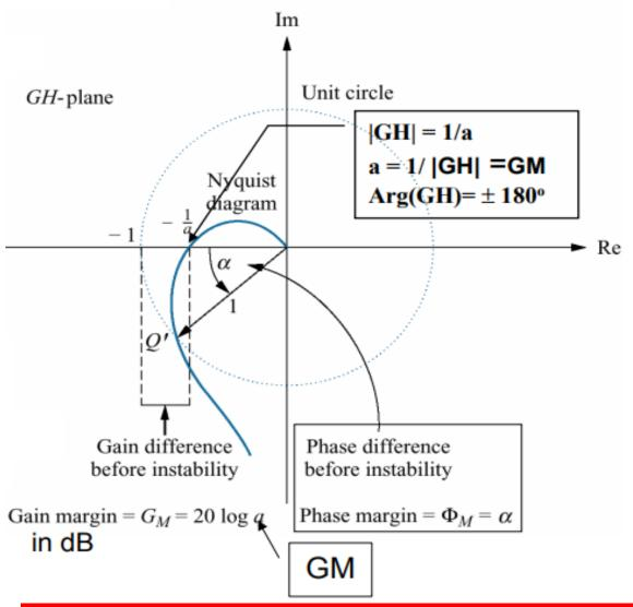
For stability, the PM must be positive. As the PM approaches 0 degrees, the system becomes more oscillatory
