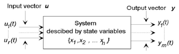
The state variables are an internal description of the system which completely characterize the system state at any time t, and from which any output variables yi(t) may be computed.
