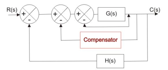
**Load Compensator** -- A compensating network is one which makes some adjustments in order to make up for deficiencies in the system.
