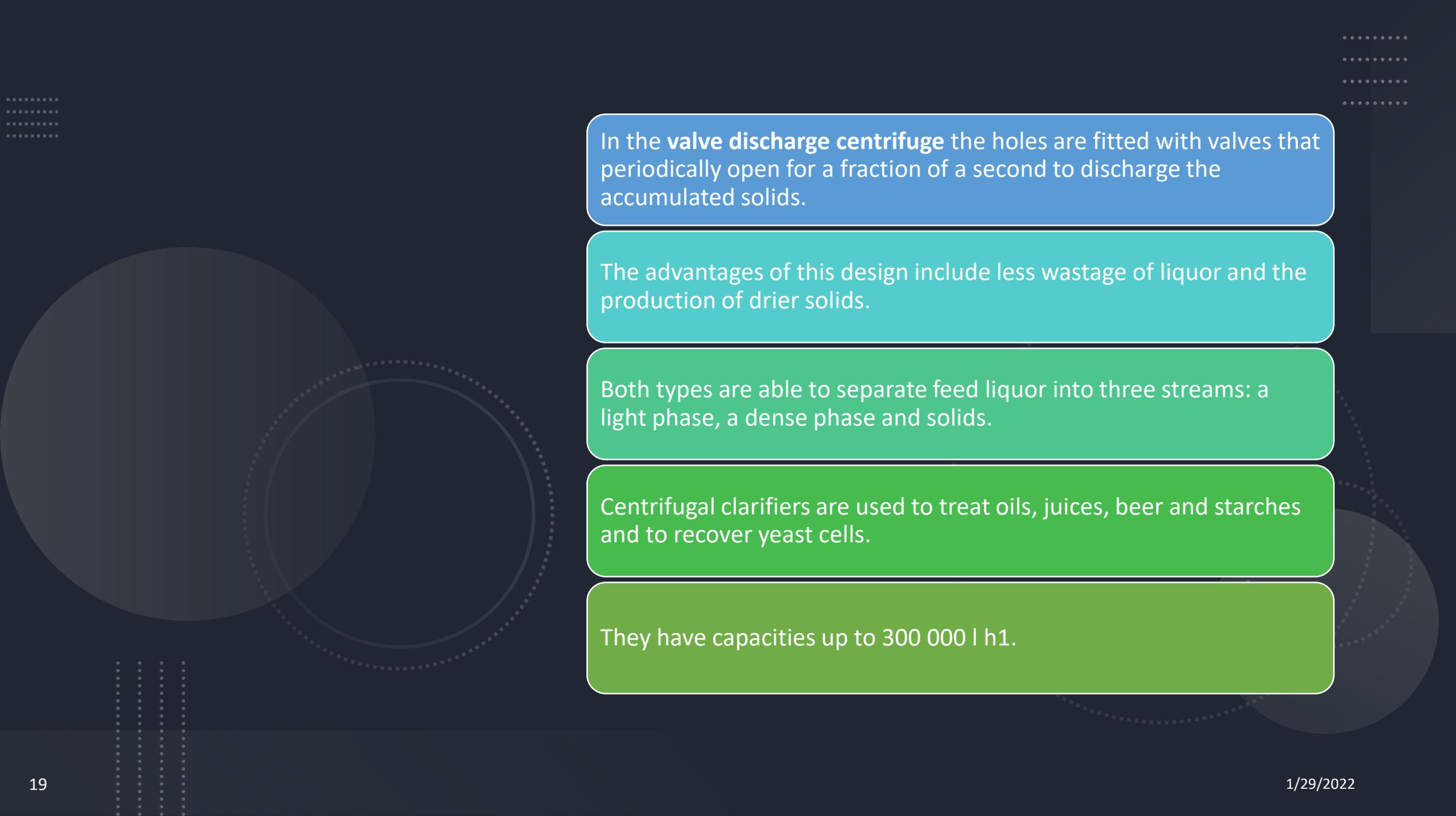
In the **valve discharge centrifuge** the holes are fitted with valves that periodically open for a fraction of a second to discharge the accumulated solids.
