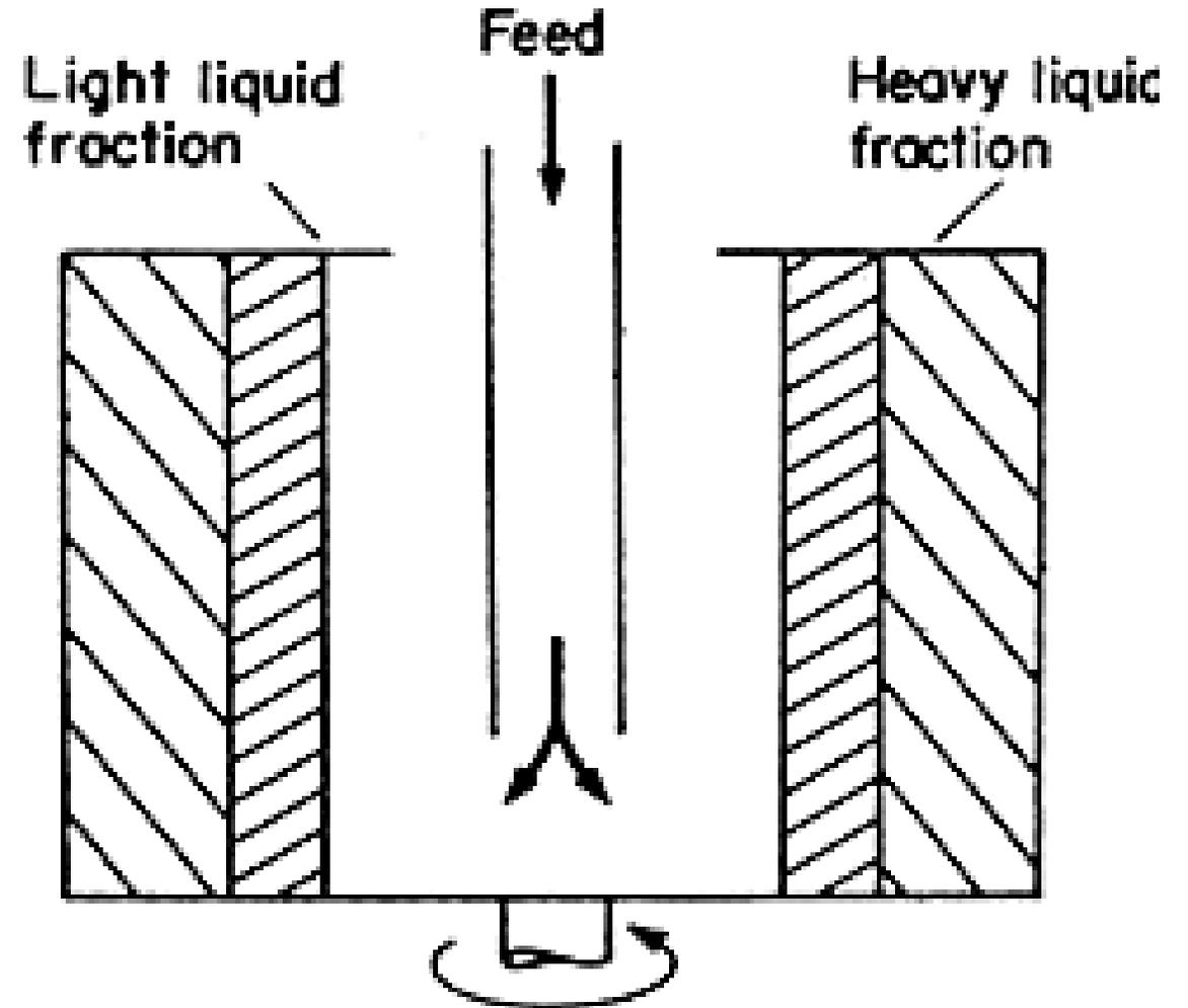
A boundary region between the liquids at a given centrifuge speed forms at a radius  $r_n$  where the hydrostatic pressure of the two layers is equal. This is termed the **neutral zone** and is important in equipment design to determine the **position of feed and discharge pipes**. It is found using:
