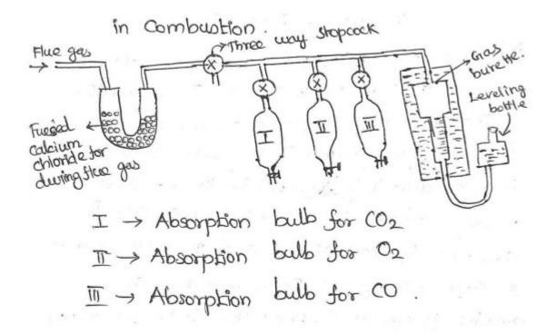
**Apparatus:** It consists a horizontal tube. At one end this tube, U tube containing fused  $CaCl_2$  is connected through 3 way stop cock. The other end is connected with a graduated burette. The horizontal tube is also connected with 3 different absorption bulbs I, II, III for absorbing CO<sub>2</sub>, CO and O<sub>2</sub>.
