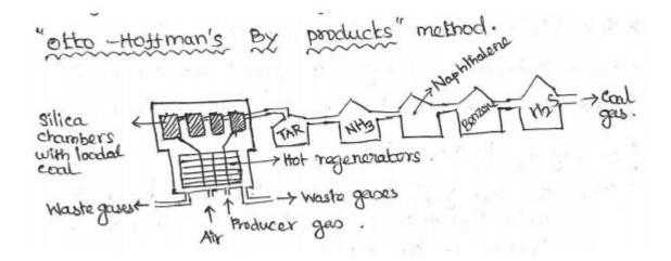
In order to (i) Increase the thermal efficiency of the carbonization process & (ii) Recover the valuable by products by this method.
