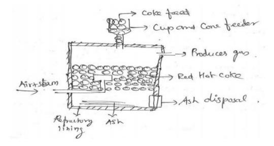
The producer gas producer consists of a tall steel vessel, lined inside with refractory bricks. It is provided with cup & cone feeder at the top & side opening for producer gas exit.
