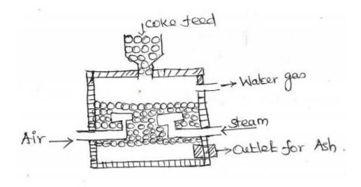
The water gas producer consists of a tall steel vessel, lined with refractory bricks.
