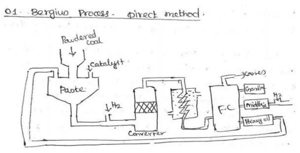
Input : Powdered coal + Ni Oleate catalyst + Heavy oil are made into paste +  $H_2$ Heating in : 400 - 450°C.
