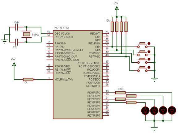
In the circuit there are 4 buttons and 4 LEDs, when a button is pressed or depressed an interrupt occurred and the microcontroller executes the interrupt routine which turn ON or OFF an LED as shown in the video below.
