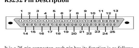
It is a 25-pin connector, each pin has its function is as follows.
