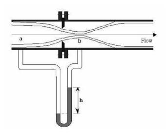
The reduction of the cross section of the flowing stream in passing through the orifice increases the velocity head at the expense of the pressure head, and manometer measures the reduction in pressure between the taps.
