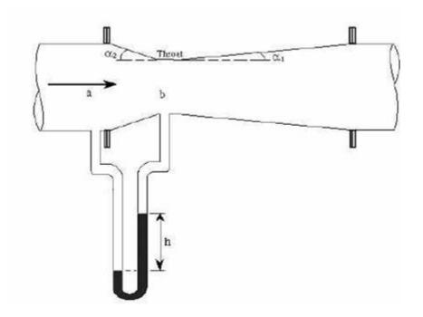
The attraction of this meter lies in its high-energy recovery so that it may be used where only a small pressure head is available, though its construction is expensive.
