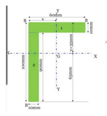
Fig. shows an unequal angle of dimensions 100mm by 60mm and 10mm thick. Determine:
