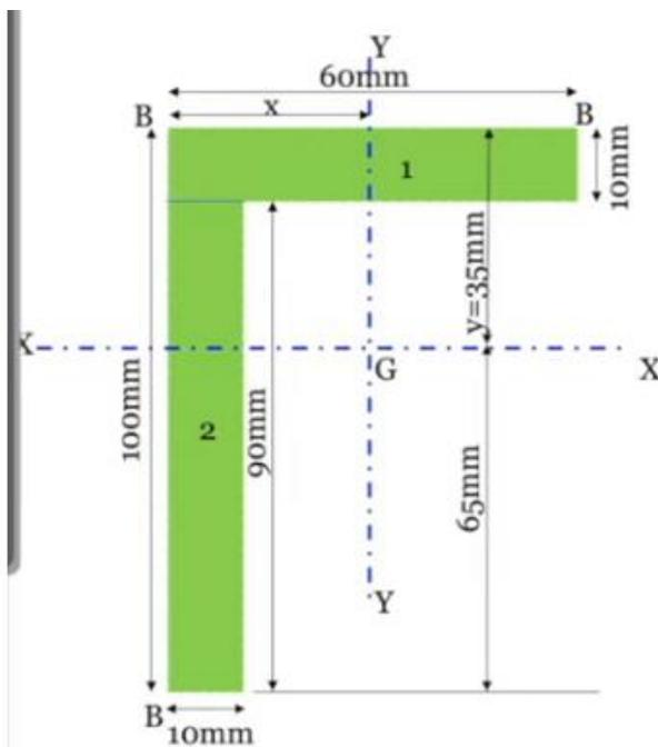
Fig. shows an unequal angle of dimensions 100mm by 60mm and 10mm thick. Determine:
