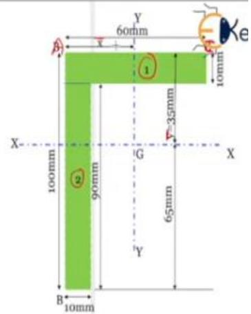
$$I_{xx} = \frac{60 \times 10^3}{12} + (60 \times 10) \times \left( \bar{y} - \frac{10}{2} \right)^2 + \frac{10 \times 90^3}{12} + 10 \times 90 \times (65 - 45)^2$$
