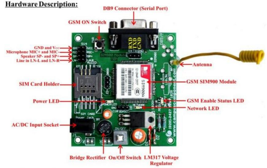
SIM900A will typically be available in modules with breakout pins for easy interfacing along with connectors for SIM cards, antennas and a few more extra features. For this guide, we will be using the AE GSM SIM900A module.
