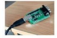
Connect three Single Berg Wires to CP2102 modules's RXD, TXD and GND pin. Then connect RXD wire to TXD of GSM module and TXD wire to RXD of GSM module. Make GND common by connecting GND wire to GND pin of GSM module.
