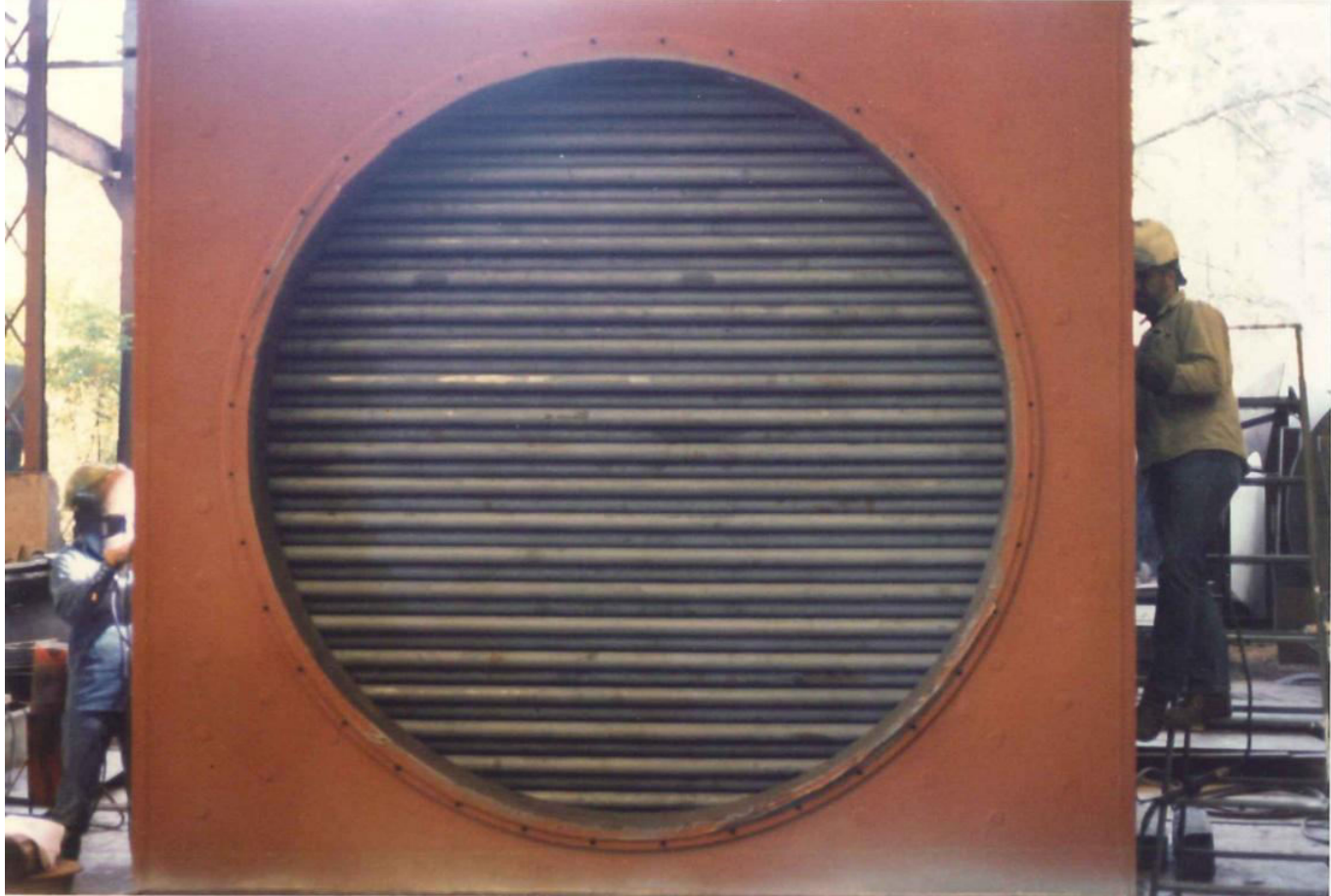
The Inlet of H 2 's Cross Flow, Staggered Tube Heat Exchanger
