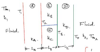
$$\frac{1}{R_{\text{parallel}}} = \frac{1}{R_{\text{R}}} + \frac{1}{R_{\text{C}}} = \frac{R_{\text{R}} + R_{\text{C}}}{R_{\text{R}} \times R_{\text{C}}} \rightarrow \frac{R_{\text{R}} = \frac{L_{\text{R}}}{K_{\text{R}} A_{\text{R}}}}{R_{\text{C}} \times R_{\text{C}}}$$
