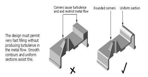
Solidification issues: Sections with different thicknesses solidify at different rates, leading to differential shrinkage and residual stresses. This can cause distortion, warping, or cracking in the casting.
