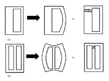
Cooling non-uniformity: Thin sections tend to cool more rapidly than thicker sections, leading to non-uniform cooling rates across the part. This can result in internal stresses, warping, and even cracking.
