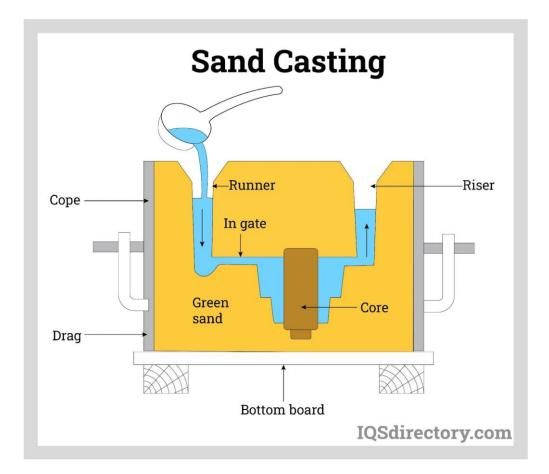
Parts manufactured using sand casting come in a wide range of sizes and weights and have complex geometries using a variety of metals. The use of sand as the casting material significantly reduces the cost of the casting process. In the metal mold process, the machining of the molds accounts for a large portion of the costs.
