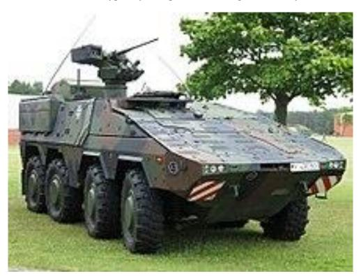
Gun carrier and transport vehicle is typically designed to protect against small arms and artillery fire. Some designs have more protection. Armour is usually composed of steel or aluminium. They will also use bulletproof glass. They are equipped
