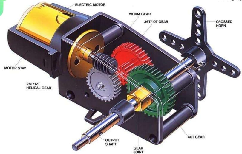
**Construction of Servo Motor**
