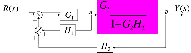
2. Moving pickoff point A behind block  $\frac{G_2}{1+G_2H_2}$
