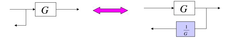
5. Moving a pickoff point ahead of a block
