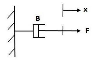
$F_{b} \propto v$   $F_{b} = Bv = B\frac{dx}{dt}$   $F = F_{b} = B\frac{dx}{dt}$
