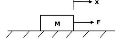
Where, **F** is the applied force  $\mathbf{F}_{\mathbf{m}}$  is the opposing force due to mass **M** is mass **a** is acceleration **x** is displacement
