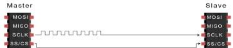
Slave select pin shifts from high to low
