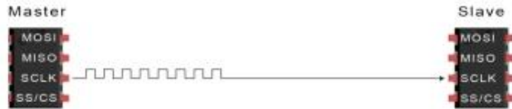
master initiates clock signal
