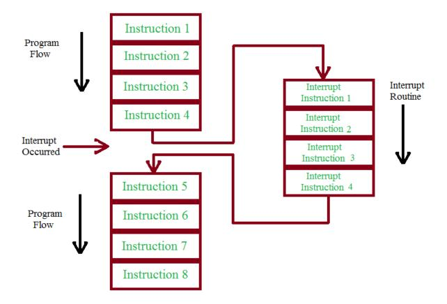
In the event of an interrupt, the source of the interrupt (like a Timer, Counter etc.) sends a special request to the processor called Interrupt Request (IRQ) in order to run a special piece of code. The special code or function is called as Interrupt Service Routine (ISR)
