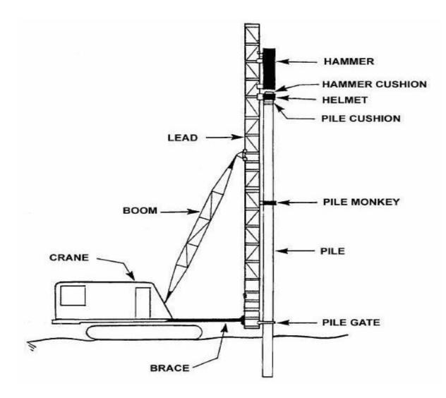
Since the air/steam hammer is an external combustion hammer, its performance depends on the boiler (steam generator) or air compressor. Either unit must be of sufficient capacity to provide the operating pressures at the necessary fluid flow rate. The hammer
