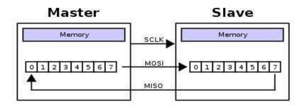
Master shifts out data to Slave, and shift in data from Slave <u>http://upload.wikimedia.org/wikipedia/commons/thumb/b/bb/SPI 8-</u> bit\_circular\_transfer.svg/400px-SPI\_8-bit\_circular\_transfer.svg.png
