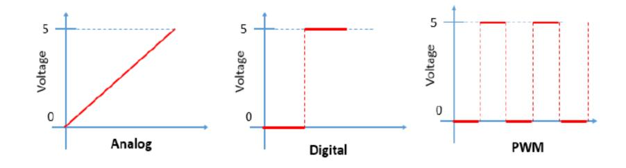
Difference between Analog, Digital and PWM Pins
