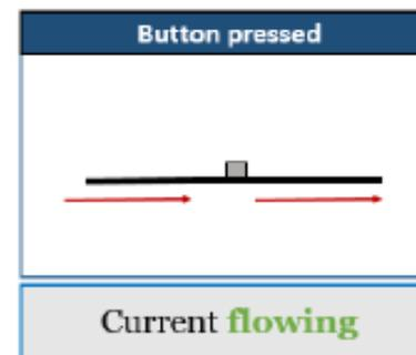
Here an **open pushbutton** mechanism is used. In Normal state(not pushed) of the button current doesn't flow, only when button is pushed flow of current is allowed
