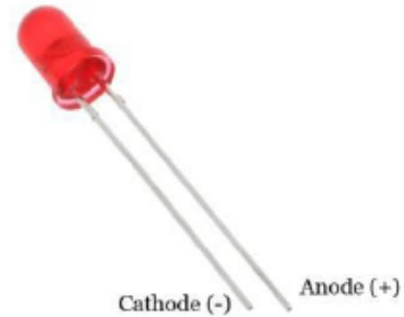
The longest lead is the anode and the shortest is the cathode.
