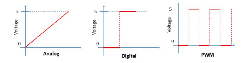
Difference between Analog, Digital and PWM Pins
