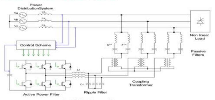
Fig. Hybrid Active power filter
