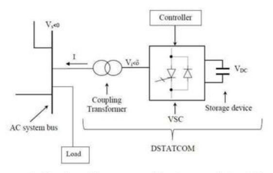
The VSC converts the dc voltage across the storage device into a set of three-phase ac output voltages. These voltages are in phase and coupled with the ac system through the coupling transformer. Such configuration allows the device to absorb or generate controllable active and reactive power.
