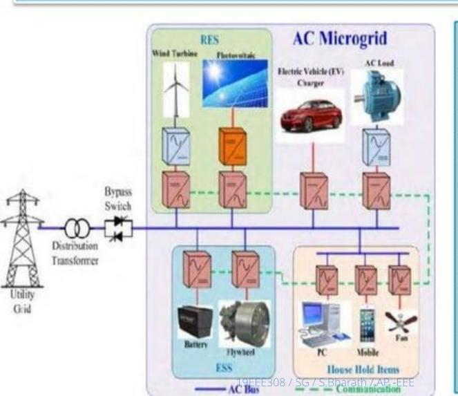
✓ An AC microgrid connects to the distribution network via an AC bus
