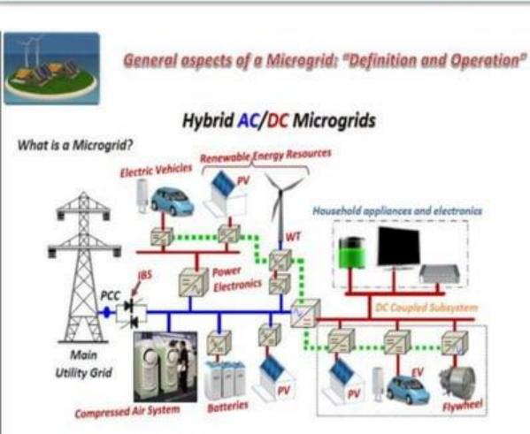
✓ An AC/DC hybrid microgrid is a microgrid consisting of an AC bus and a DC bus
