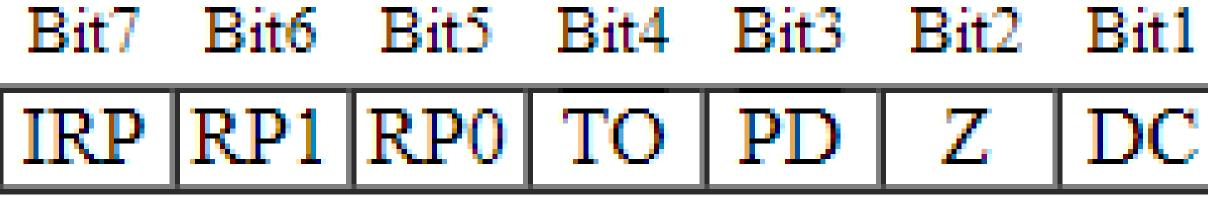
► If the STATUS register is the destination for an instruction that affects the Z, DC or C bits, then the write to these three bits is disabled.
