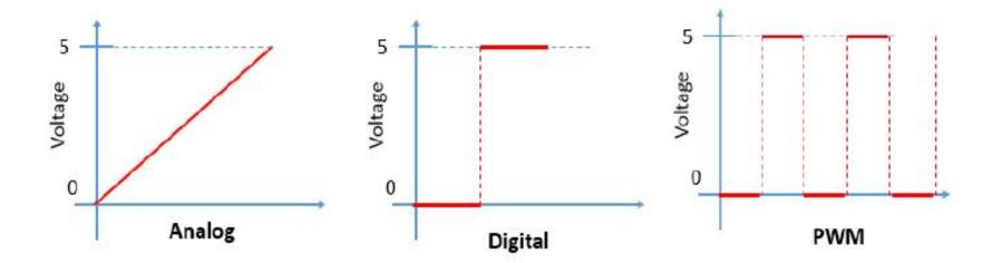
Difference between Analog, Digital and PWM Pins
