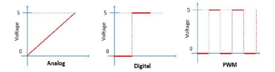
Difference between Analog, Digital and PWM Pins
