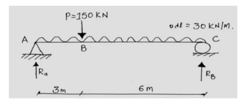
Determine the vertical deflection at point 150KN load in fig.
