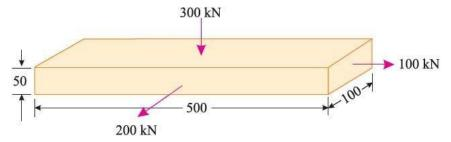
Given Data: Length (l) = 500 mm; Width (b) = 100 mm; Thickness (t) = 50 mm;
