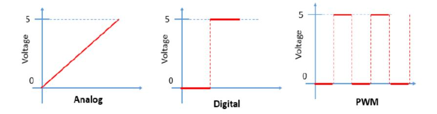
Difference between Analog, Digital and PWM Pins
