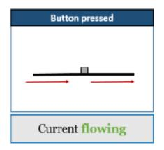
Here an **open pushbutton** mechanism is used. In Normal state(not pushed) of the button current doesn't flow, only when button is pushed flow of current is allowed
