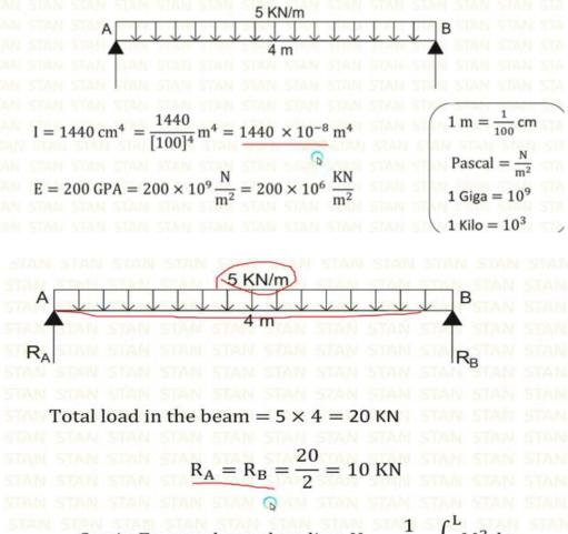
Strain Energy due to bending,  $U = \frac{1}{2EI} \int_0^L M^2 dx$
