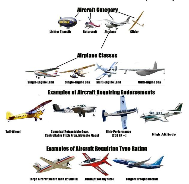
Aircraft can be categorized into various types based on their design, purpose, and mode of operation. Here are some of the different types of aircraft:
